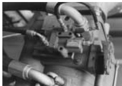
An RPA can be direct mounted to control the output of a variable displacement pump.
